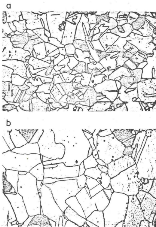
FIG. 5. Microstructures of copper after shock loading at 500° (a) and 400° (b). Cooling in water; \times 100 .
